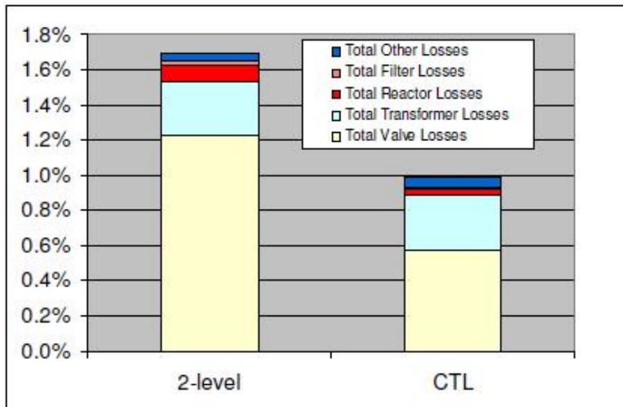
**Figure 12.** Vertical bar graph for comparison of losses before technique & after using technique
