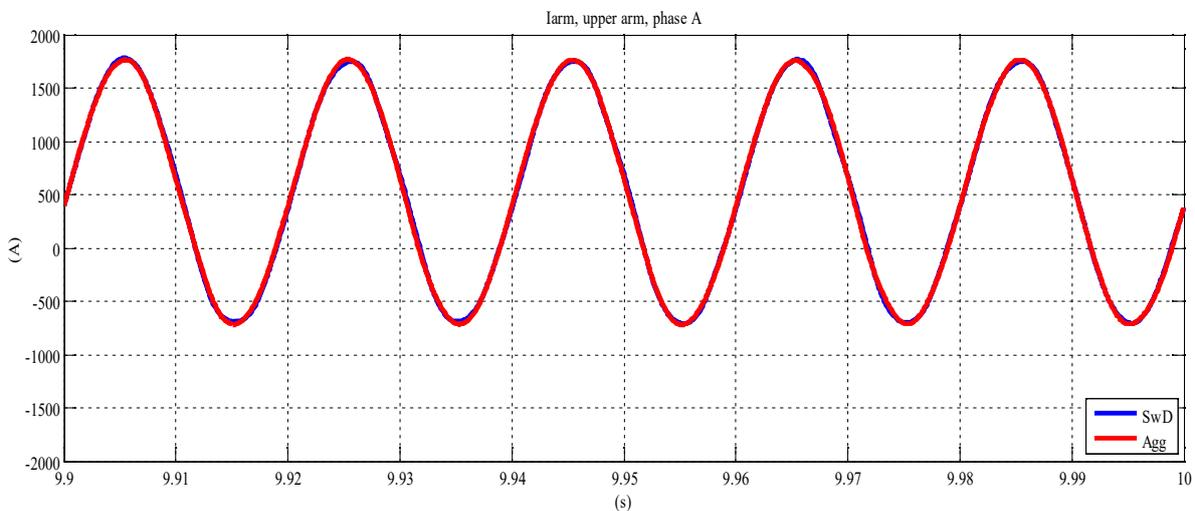
**Figure 10.** Upper arm current of phase line ‘A’
